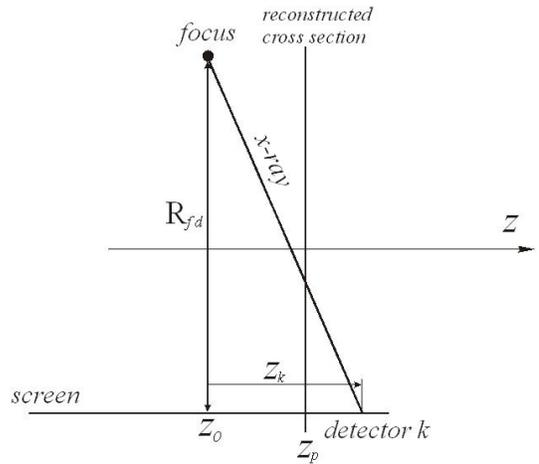
Fig. 2. The geometry of the cosine correction factor
